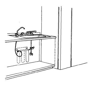
3. Or, install faucet in sink and connect blue tubing to filtration assembly. (Steps 2d-2g)
