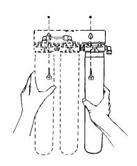
1. Slide filtration assembly onto mounting screws. (Steps 3a-3c)
