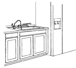
4. If filtration assembly was connected to sink faucet, lift faucet handle to discard 2-3 gallons of water. (Step 3f)
