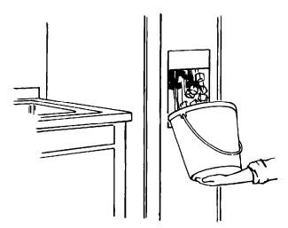
3. If filtration assembly was connected to refrigerator, make and discard 2 batches of ice and drain2-3 gallons of water from water dispenser. (Step 3e)
