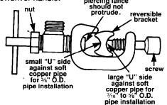
Assemble saddle valve on copper pipe. Assemble saddle valve on top side of horizontal pipe or side of vertical pipe to keep sediment from collecting in its valve.
