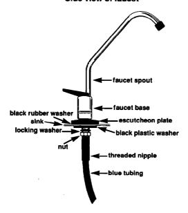
Recheck faucet position. If position needs minor adjusting, wrap the flat chrome sides of faucet and the crescent portion of the crescent wrench with masking tape to protect the chrome from scratches. Use the wrench on flat sides of faucet to reposition faucet. Remove masking tape.
