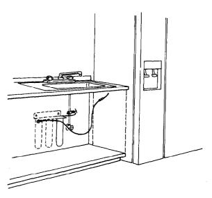
2. Connect refrigerator's water supply to filtration assembly with blue tubing. (Steps 2b-2c)
